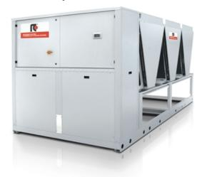
Outdoor unit for the production of chilled water with hermetic rotary Scroll compressors, low-GWP and ozone-friendly refrigerant R454B, axial-flow fans, braze-welded plate-type heat exchanger, micro-channel full-aluminum air coils and thermostatic expansion valve. The range is composed by units equipped with four compressors in tandem configuration on two independent refrigeration circuits.
